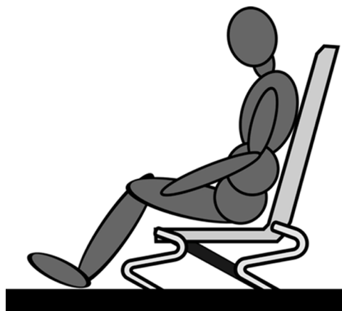
Figure 8 Energy absorbing seat with S-shape legs
