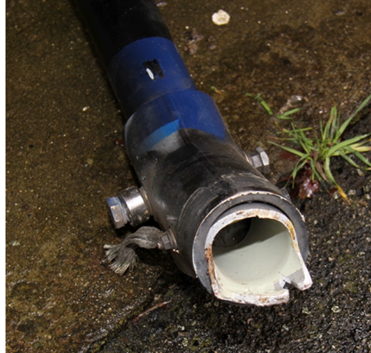
Figure 3 Crosstube break off point (see online version for colours)
