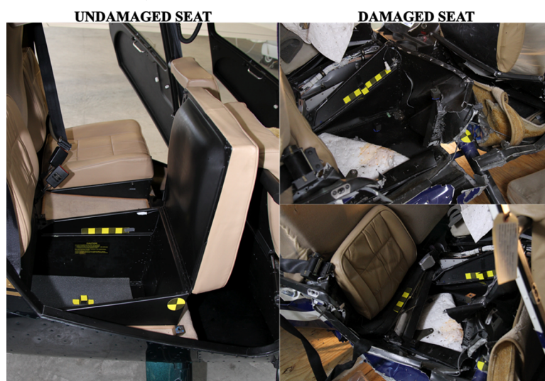
Figure 2 Rear right seat comparison from undamaged to post-incident (damaged) (see online version for colours)
