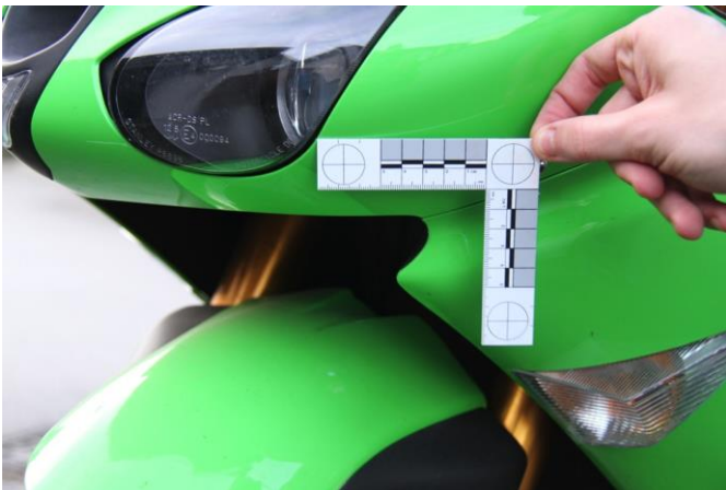
Figure 5: Notch on the left side of the front fender of the 2008 Kawasaki Ninja ZX-6R inspected during the full-scale motorcycle examination.
