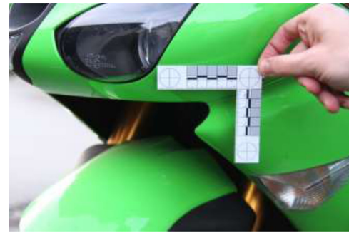
Fig. 5. Notch on the left side of the front fender of the 2008 Kawasaki Ninja ZX-6R inspected during the full-scale motorcycle examination.
