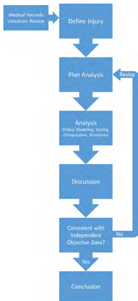
Figure 2. Workflow diagram for injury reconstruction
