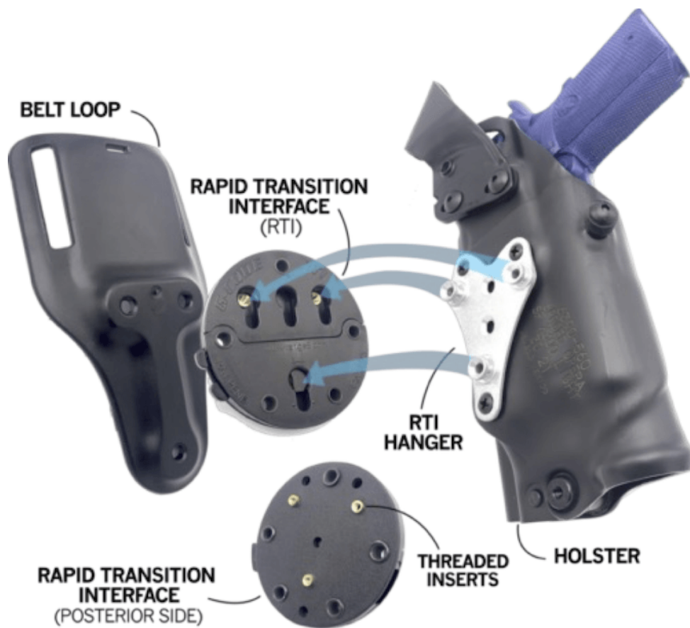
Figure 1 Rapid Transition Interface RTI Wheel <br>Image courtesy of GTD Scientific
