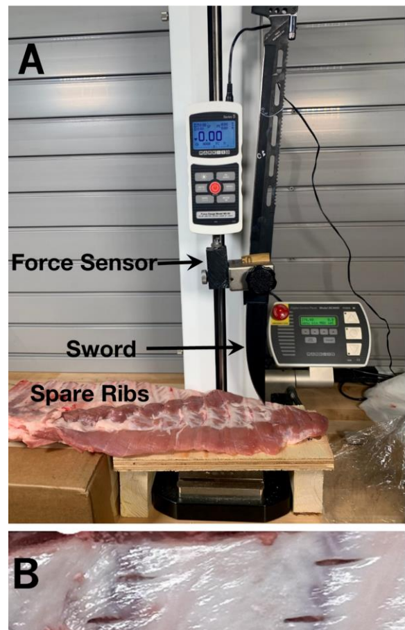
Fig. (2). (A) MK-10 Tensile Tester shown with clamped ceremonial sword, illustrating position of sword tip prior to penetration of pork rib cut. (B) Example of four penetration wounds where each parallel pair represents a penetration at 350 mm/min and a penetration at 1100 mm/min. (A higher resolution/colour version of this figure is available in the electronic copy of the article).
