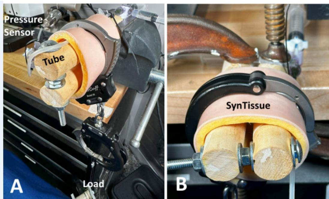
**Figure 1:** (A) Experimental setup for measuring pressure when loading the handcuff. Weights are suspended from a cable looped through the loose manacle; (B) Experimental setup for measuring pressure when tightening the handcuff.
