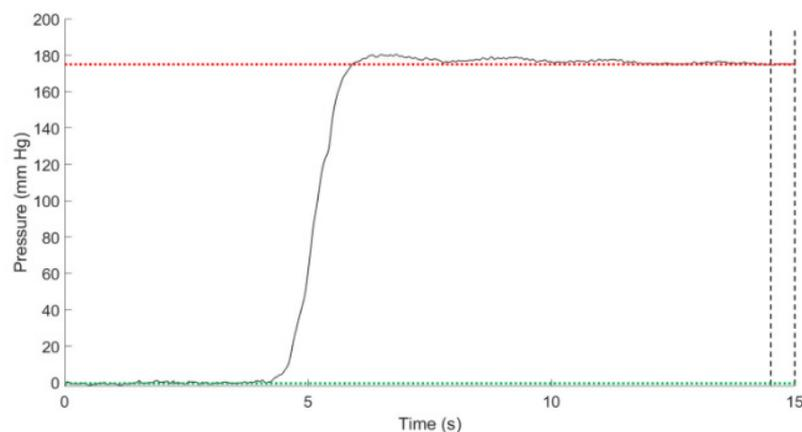
**Figure 3:** Pressure measurement from a trial with a 5 lb load suspended from the ASP handcuff. Horizontal green dotted line indicates baseline pressure and vertical dashed black lines indicate 0.5 s time interval for calculating average pressure. Pressure due to the load is the difference between the red and green dotted lines.
