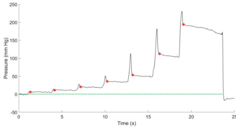
**Figure 4:** Pressure measurement from a trial in which the ASP handcuff was incrementally tightened. Horizontal green dotted line indicates baseline pressure and red asterisks indicate the pressure, immediately after the transient increase pressure as the strand was tightened by one ratchet tooth. Pressure due to tightening is the difference between the pressure at the red asterisk and the green dotted line.
