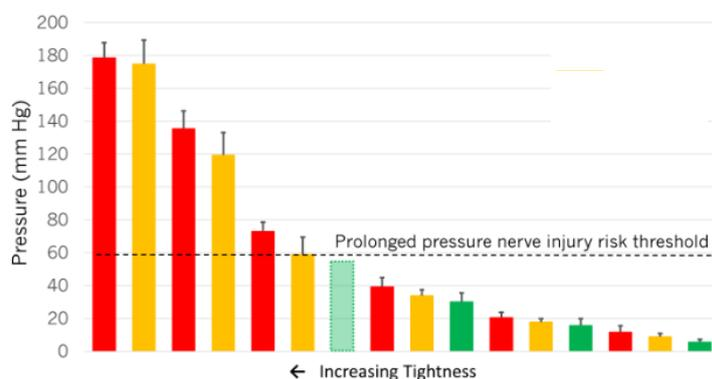
**Figure 7:** Mean pressure for 5 trials as tightness was incrementally increased, displayed with standard deviation, for the three handcuffs. The pale green bar outlined with dotted lines indicates the predicted pressure for the Spider Cuff had it been possible to tighten the strand by an additional increment.
