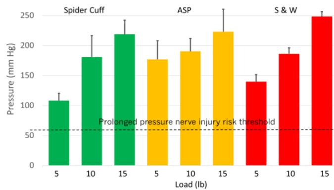
**Figure 5:** Mean pressure for 5 trials, displayed with the standard deviation, for each load for the Spider Cuff (■) ASP handcuff (■) and Smith and Wesson handcuff (■). The dashed horizontal line indicates the threshold for risk of nerve injury when constant pressure is maintained for at least 1 h.
