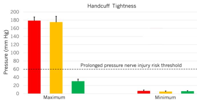
**Figure 6:** Mean pressure for 5 trials, displayed with the standard deviation, for the minimum tightness at which pressure first began to increase above the baseline level (right) and for the maximum tightness that could be achieved (left) for the three handcuffs.
