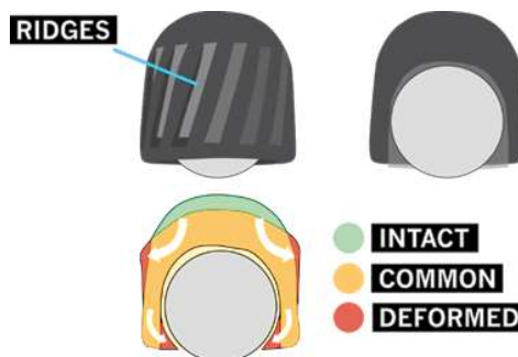
Figure 9: Deformation of 12-gauge slug.
