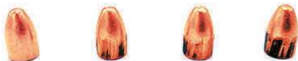
Figure 3: Intact 9mm bullet (left) compared to three (3) fired and captured 9mm bullets.
