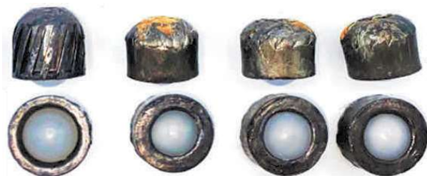
Figure 8: Intact 12-gauge slugs (left) compared to three (3) fired and captured 12-gauge slugs.
