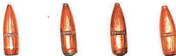
Figure 6: Intact .223 Remington bullet (left) compared to three (3) tested .223 Remington bullets.
