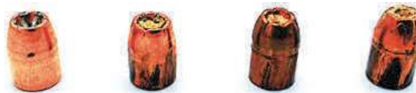
Figure 5: Intact .40 S&W 165Gr bullet (left) compared to one (1) intact 165Gr and two (2) 180Gr (right) fired and captured bullets.
