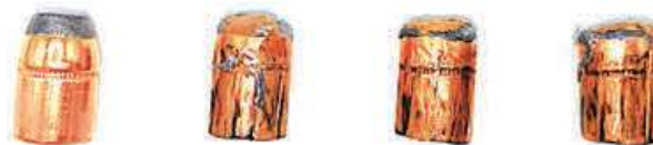
Figure 7: Intact .44 Magnum bullet (left) compared to three (3) fired and captured .44 Magnum bullets.
