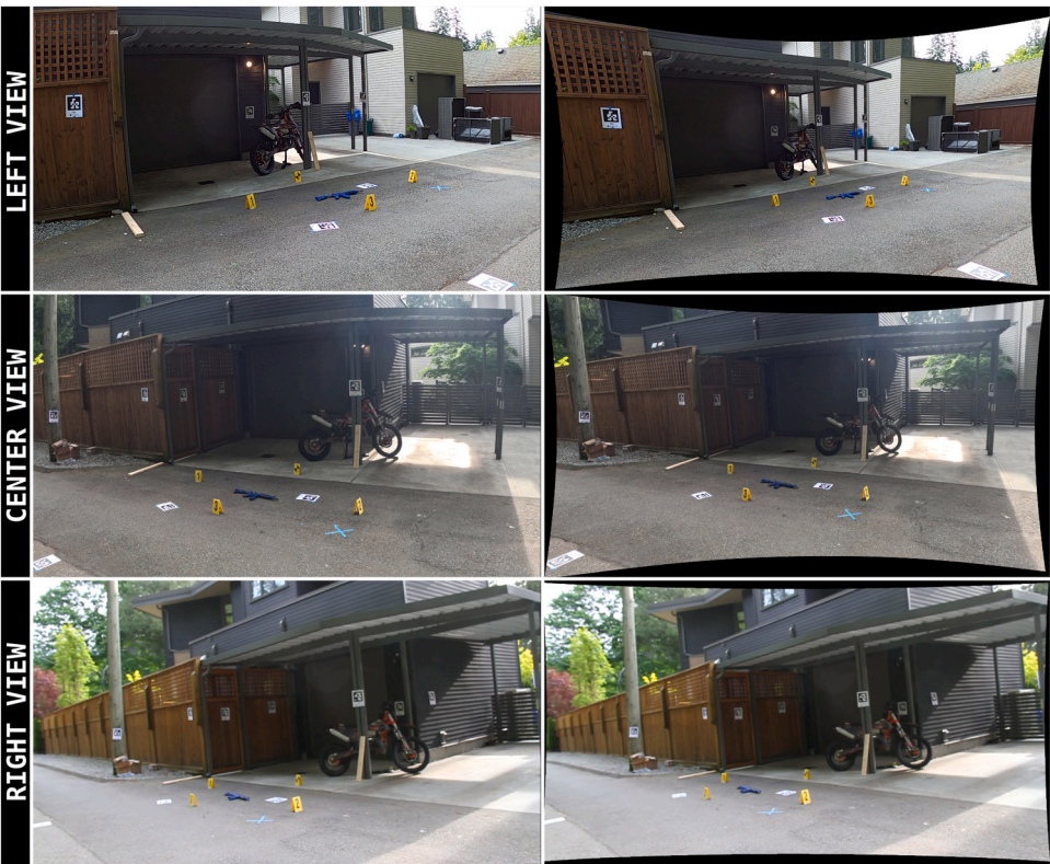
Fig. 1. Frames from camera views of simulated forensic incident scene as recorded on the left and the same frames after lens correction for distortion in Photo-modeler on the right.
