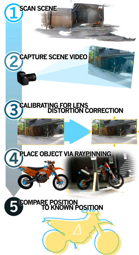
Fig. 1. Illustration of the steps involved in calculating the error between the true position of an object and its calculated position based on photogrammetry using the method of ray pinning.
