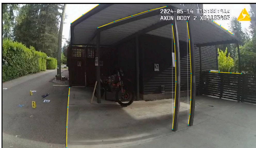
Fig. 14. The uncorrected image with the lines which would be used to perform the straight-line correction, of which the result can be seen in Figs. 12 and 13. Note the lack of contrast between the vertical beams and building wall, the shadowing effect near the garage door, and the low resolution of the fence on the right-middle side of the image.
